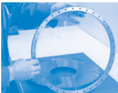
8: Clean and degrease upper clamping ring.
