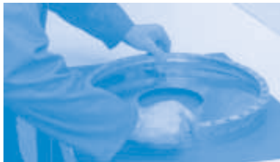
9: Match up balance marks of clamping rings and place upper clamping ring properly aligned on top of blade and lower clamping ring.
