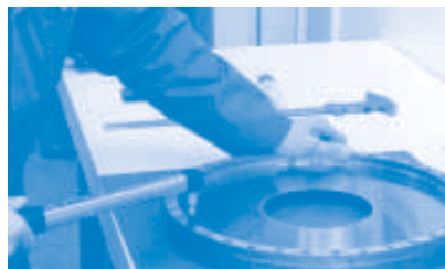
Tighten clamping screws crosswise using an Allen wrench. Generally the clamping ring screws (M6 property class 12.9) are tightened with a torque wrench to 15 Nm. To avoid screw failure, screws should be replaced at every blade change.
