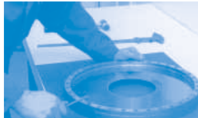
10: Place screws into clamping rings and tighten screws hand-tight.
