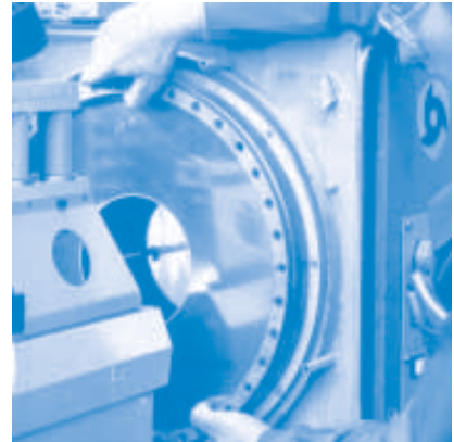
13: Mount clamping rings with saw blade on top of tensioning ring.
